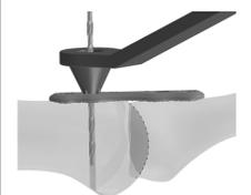
7. Select desired screw diameter to use and corresponding pilot drill.
